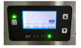
An advanced graphical display monitors the status of each filter and when they need to be replaced an LED lights up. A calibrated VOC/gas sensor is used to monitor filter effectiveness. Electronic four speed blower control is used to optimize source capture in your operation and with your materials.
