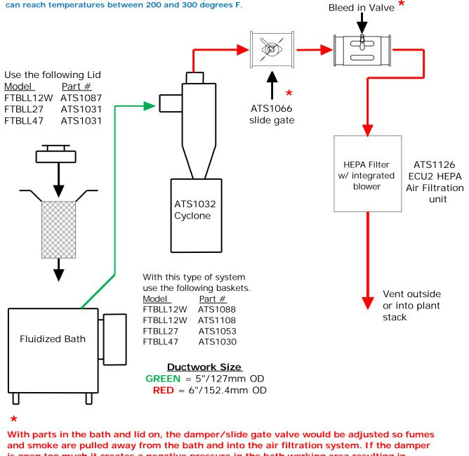
and smoke are pulled away from the bath and into the air filtration system. If the damper is open too much it creates a negative pressure in the bath working area resulting in significant heat and sand loss. The purpose of the Cyclone is to recover any sand pulled out and heavier deposits which can be sieved and reused. The bleed in valve is opened to cool down the exhaust air stream before entering the filtration unit.
