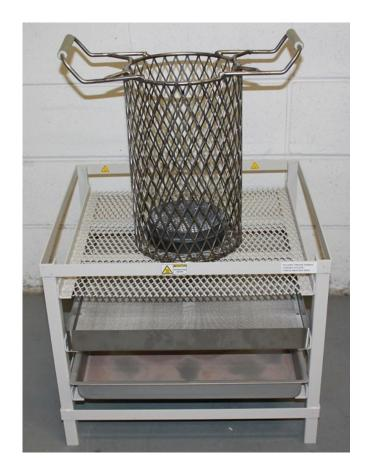
The cooling stand and sieve was designed to allow the operator who is cleaning tooling to safely locate the very hot parts basket out of the way. Its secondary role is to capture any ash and carbon residue from the plastic in the sieve which allows reusable aluminum oxide sand to fall into the catch pan. This accessory keeps the work area cleaner and safer as well as allowing for the reclaim and reuse of aluminum oxide sand.
