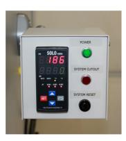
The model FTBLL27 and FTBLL47 use a PID temperature controller that has four control zones for improved thermal results. Independent over temperature protection will disable heat if the temperature exceeds 610°C or if the air supply pressure drops below 60 PSI. Fluidizing air is automatically controlled by the system. The remote control box includes an RS485 computer interface for connection to a PC with downloadable software from our website.
