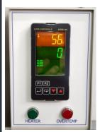
All of our Fluidized Baths use a temperature controller that has four PID control zones for improved thermal results. Independent over temperature protection will disable heat if the temperature exceeds 1140°F or in the event of a system failure. The systems are double fused for improved safety and include an RS485 computer interface for connection to a PC.
