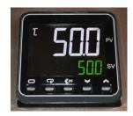
The ThermCal130 controller offers a large, bright and easy to read display. The unit is switchable between °F and °C along with the ability to adjust unit calibration using your own reference standard. Up to 8 set points can be saved for quick recall.
