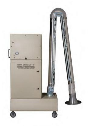
The M66 from Air Quality Engineering, Inc. is a self-contained media air cleaning system designed for use in source capture applications where mobility is desired. The M66 can be ordered in a three-stage filtration configuration which will effectively remove a broad range of airborne contaminants including fine dust, smoke, soot, vapors, mist, VOC's and more at a rate of up to 2000 CFM.
