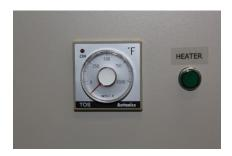
The model FTBLL12E Fluidized Temperature Bath has an easy to use dial controller for setting the bath from 100 to 1000°F. The heater light shows heater status and once flashing you allow an hour for the system to fully reach operating temperature.
