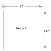
The DCS2500 has a relatively small footprint as shown but is 108" long. In the horizontal configuration it can be mounted to a wall and in the vertical configuration it can be free standing. It is ordered in either configuration that best suits your space and layout considerations. Three feet of clearance is needed on the inlet side of the system to open the filter access panels.
