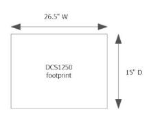
The DCS1250 has a relatively small footprint as shown and is only 55" tall. It can be mounted to the wall with the optional mounting kit or remain free standing. We recommend placing in a location that offers 4 or 5 feet of space around the unit to access the filters and for ductwork connection and maintenance.
