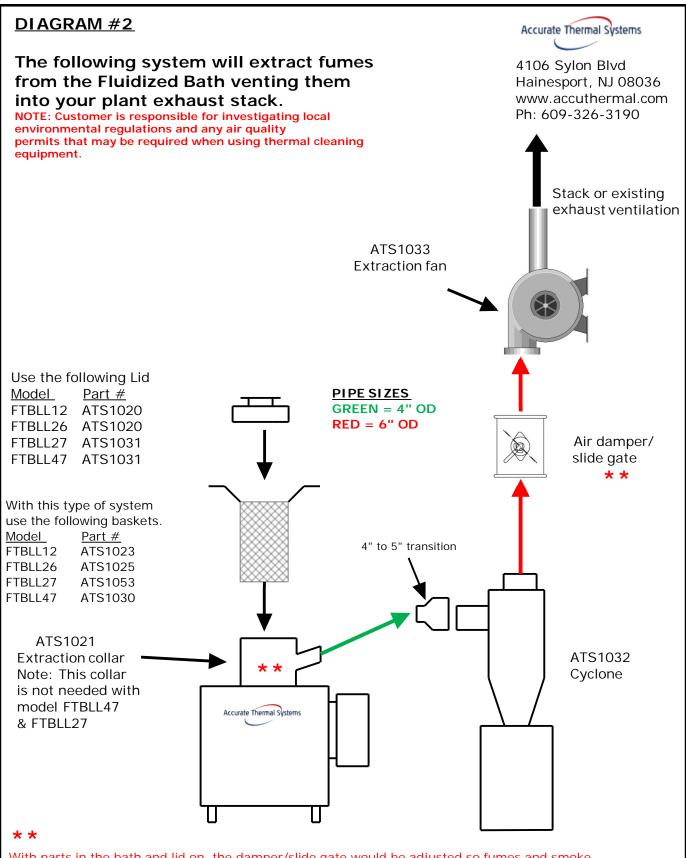
With parts in the bath and lid on, the damper/slide gate would be adjusted so fumes and smoke are pulled away from the bath and into the exhaust system. If the damper is open too much it would create a negative pressure in the bath working area resulting in significant heat and sand loss. The purpose of the Cyclone is to recover any sand pulled out and heavier deposits which can be sieved and reused.
